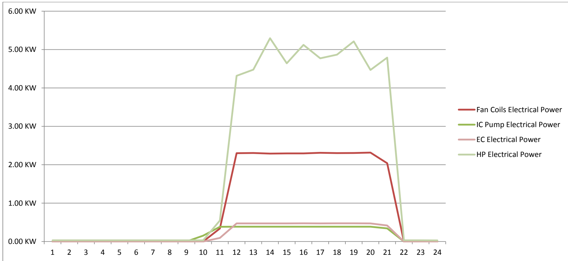
Graph4: Thermal Power (heating , cooling & sanitary hot water) delivered to the building; Thermal Power to/from the BHE; Electrical Power consumption at the compressor (heat pump); Electrical Power consumption at the external pump; Electrical Power consumption at the internal pumps; Electrical Power consumption at the fans (FCUs or AHU)
